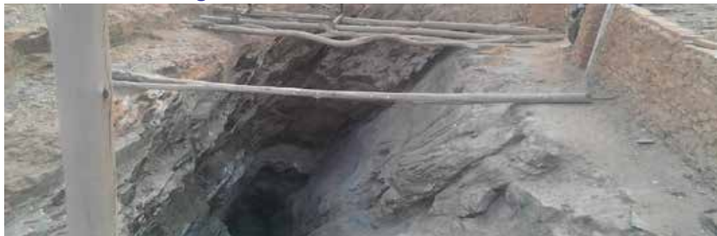
Figure 32: Example of mining method: Inclined shaft mining near Kazangarare Growth Point, Hurungwe District.
