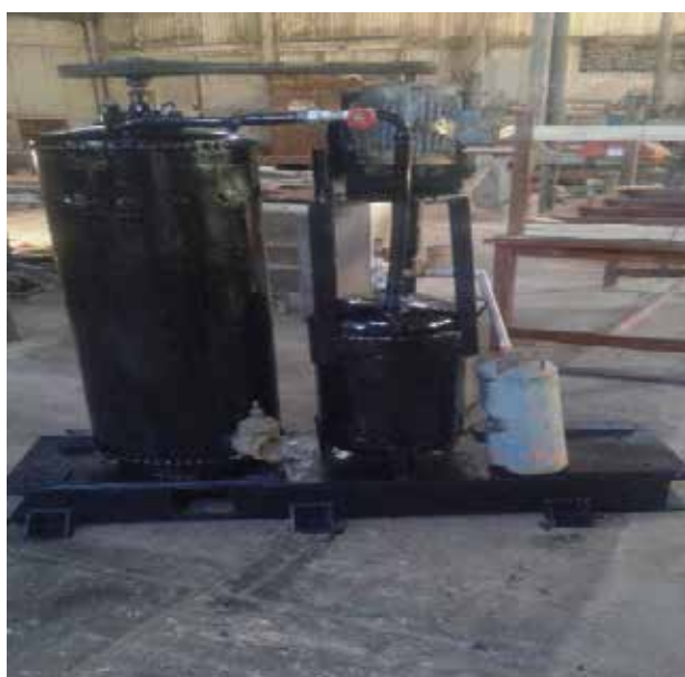
Figure 13: Prototype anaerobic digester and natural fertiliser producing reactor
